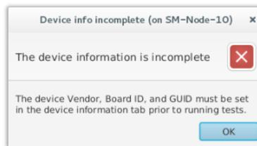
FIGURE 9 – MISSING DUT INFORMATION WARNING
